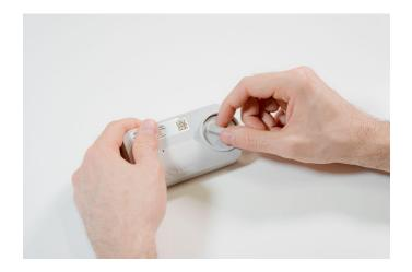
Open the connector, the beige part in the front of the device, by lifting the black lever of the connector upwards and insert the sensor with the print facing upwards.
